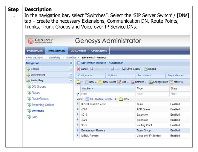
2 Extension DNs are defined for SIP endpoints (phones) that register with SIP Server. Make sure that the following options are set in the <Extension DN>/[Options] tab/TServer section (extension 4020 is used as an example):
