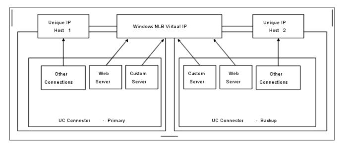
This figure shows an overview of how HA-enabled UC Connector instances can be deployed. While web communication with the UC platform uses a single Virtual IP address to communicate with UC Connector, Genesys Management and Configuration Layer components and T-Library clients use the unique IP address for communication with the UC Connector and the Local Control Agent (LCA) installed at each UC Connector host.
