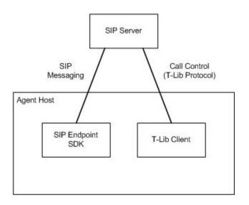
As you can see, the SIP Endpoint SDK handles the SIP messaging, and the T-Lib Client uses the T-Lib protocol to handle call control.
