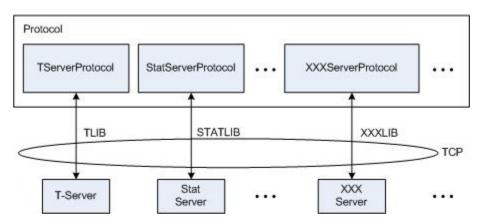
Each protocol object subclasses ClientChannel, which in turn subclasses DuplexChannel and implements the Protocol interface. This means they all share a common interface to the Genesys servers. The protocol objects communicate with the corresponding Genesys servers over a TCP connection, with each one using the native protocol of the server it connects with. For example, the TServerProtocol object communicates over TCP with a T-Server, using the TLIB protocol that is native to the T-Server.
