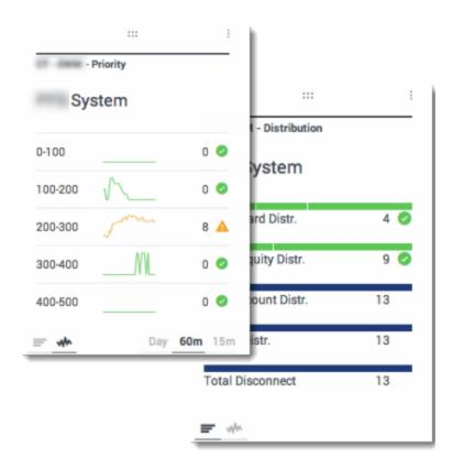
The List widget displays either one statistic for many objects or many statistics for one object. Depending on the reference selected, the Headline type option might be available for this widget type.
