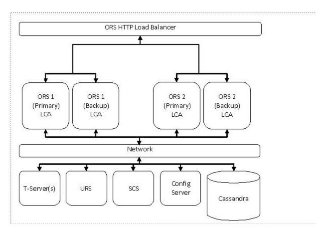
The above figure illustrates a simple two-ORS Node cluster deployment. It shows four ORS instances
