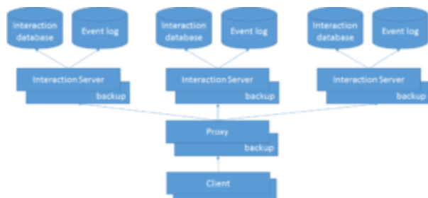
Interaction Server Cluster Deployment
