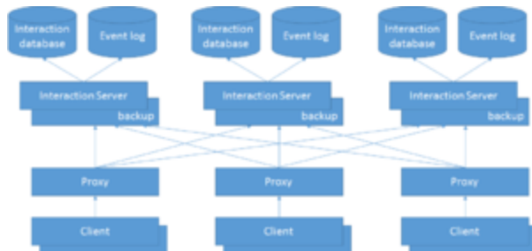
Cluster Deployment with Multiple Proxies
