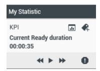
Use the **Back**, **Stop/Play**, and **Forward** buttons on the control panel to scroll manually through the statistics that you are configured to view. The buttons are displayed if you are configured to view more than one contact center statistic or KPI.
