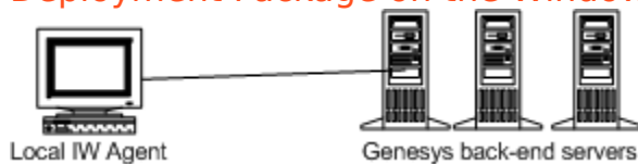
Simple client-server deployment of Workspace
