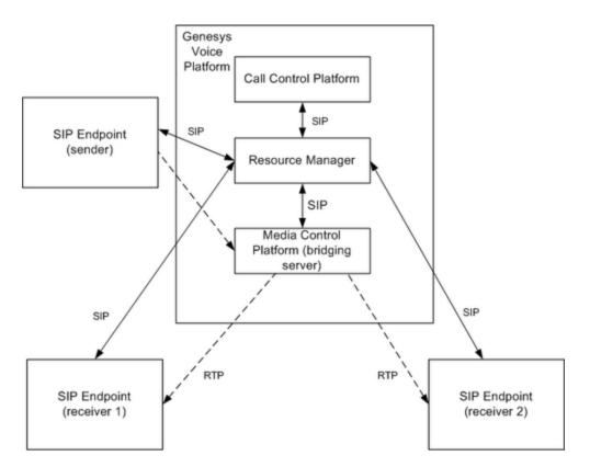
The bridging server can be accessed directly from the CCP or via the RM. The mediacontroller.bridge\_server configuration parameter is used to specify the location of the bridging server. If the bridging server is to be accessed via the RM, the location of the RM should be specified in the configuration parameter mediacontroller.bridge\_server.
