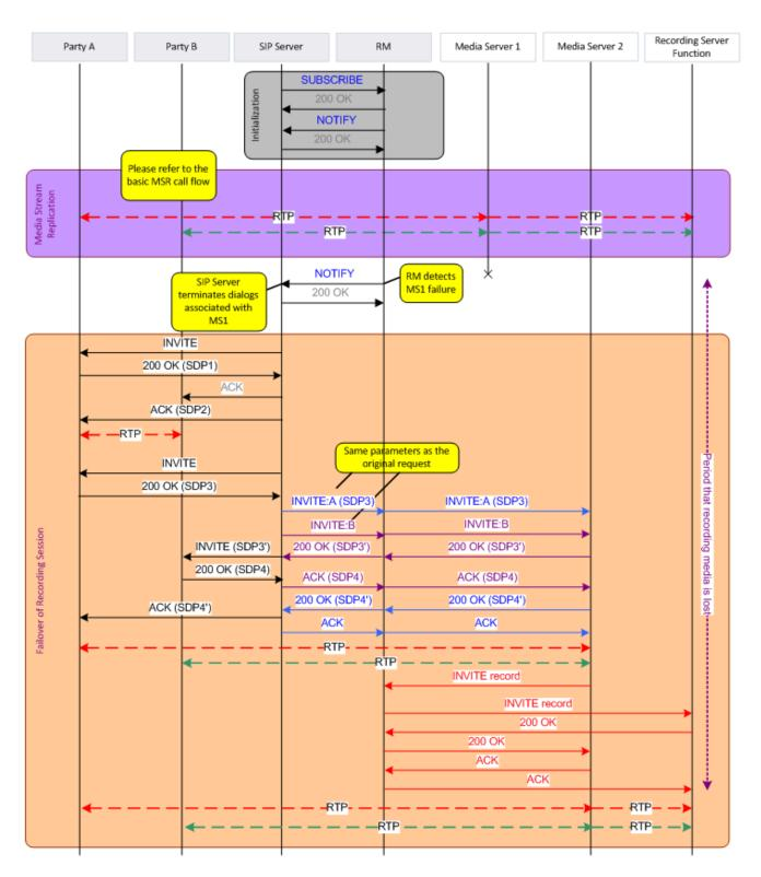
The total amount of recorded media lost is the sum of time for Resource Manager to detect MS1 failure plus the amount of time to failover the recording session to another Media Server instance.
