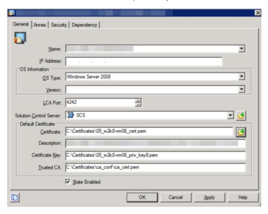
Paths to the physical certificates can be configured either on the Application or the Connection level, but not on the Host level (despite this being a general Genesys recommendation). For Host level certificates, if GRAT and GRE are located on the same host as Configuration Server or Message Server or other C++ applications, the secured connection will not be established because C++ based applications do not accept PKCS#8 format.
