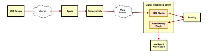
Generally, a customer enters a question, response, or similar information on their iOS device, which sends the message through the Apple Server and Genesys Hub to the Digital Messaging Server. The Routing Server then routes it through the BOT Gateway to Intelligent Automation, which forwards it on to the enterprise. To send a message back to the customer, the enterprise sends a message in a similar route, where Intelligent Automation sends it back to the customer.
