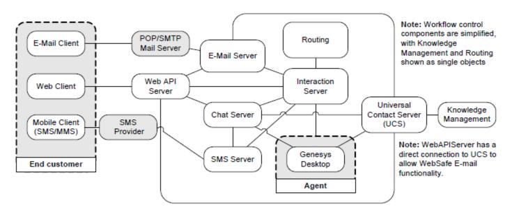
Note: Each Genesys component also connects to the Configuration Server for configuration data.
