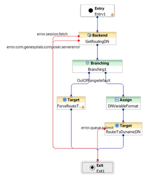
1. In the GetRoutingDN Backend block the application accesses some backend business routing logic defined in the file ../include/SomeRoutingLogic.jsp. This business logic will pass back a DN to route to in the varRoutingDNFromLogic variable.
