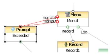
In the above example, the red links (going from the Menu block to the Prompt block) result from using the Exception Link tool to connect the two blocks. The black links (going from the Menu block to the Record block and the Log link) result from using the Outlink tool.
