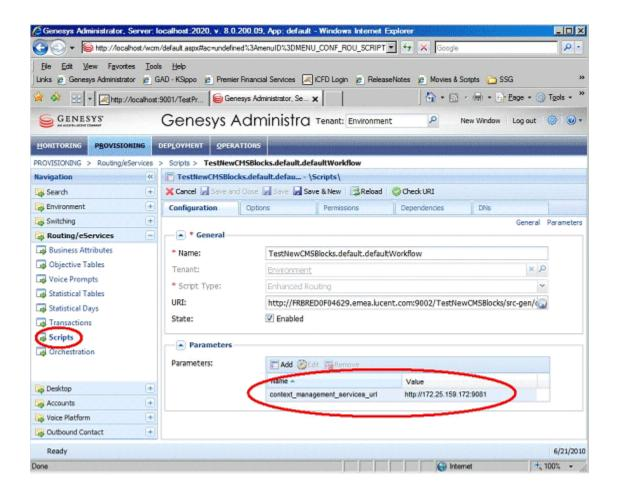
The Script objects are automatically created by Composer and the url is also automatically set if the Project is deployed within Composer (in embedded TOMCAT)
