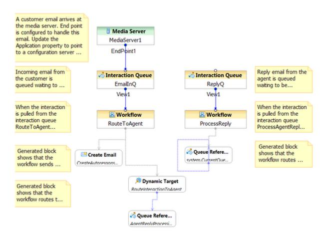
• Orchestration Server then pulls the interaction from the queue and starts processing the RouteToAgent workflow shown below.
